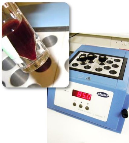
Figure 4.1 RSM verification acid hydrolysis experiments performed in a temperature-controlled heating block. Reacti-vial with dark red-brown-coloured hydrolysed C. maculata extract after hydrolysis shown.
